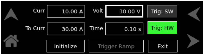
Figure 3-27. Current Ramp-Screen (HW Trigger)
