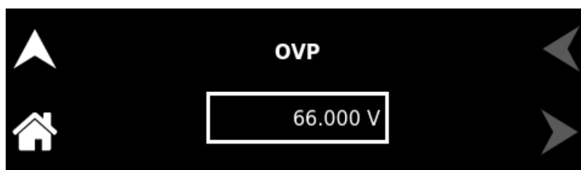
Figure 3-39. Power On OVP Setting
