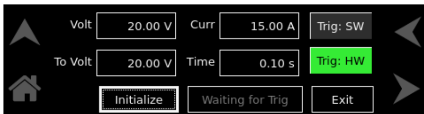
Figure 3-23. Voltage Ramp-Screen (HW Trigger)
