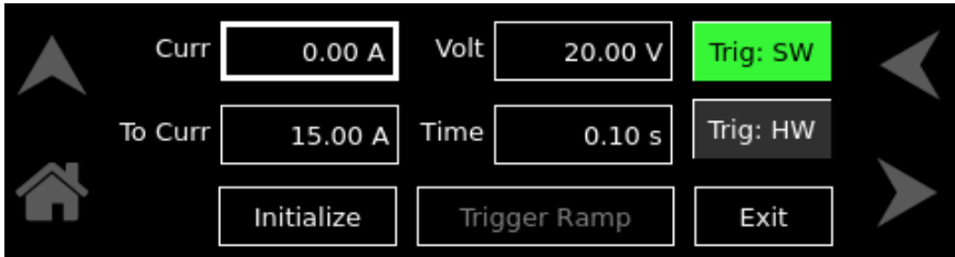
Figure 3-26. Current Ramp-Screen (SW Trigger)
