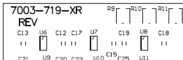
Figure 8-1. AUX Generator PWA Potentiometer, R9
